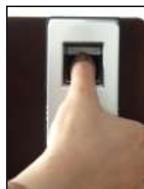
③ Put fingerprint on the scanning window, when hearing a beep, reposition the finger to scan the second fingerprint. Once success, hearing 2 prompt beeps, LED displays 02.
